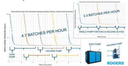
Following this tack, we've now created the familiar scenario where there is an "Evacuation Pump" performing the 'hog-down' of the process vessel with a secondary "Holding Pump" doing the job of maintaining the low pressure set point required by the process for the duration of the batch cycle.
