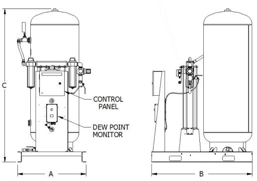
The desiccant dryer includes pre and after filters, regulator with gauge, safety valve and an isolation ball valve.
