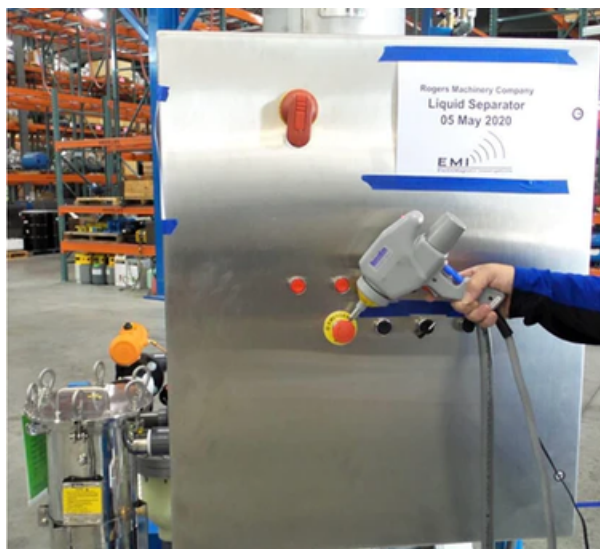
Figure 9: Electrostatic discharge testing of a Rogers Vacuum System verified that static discharges up to 8kV will not disturb our equipment operation.
