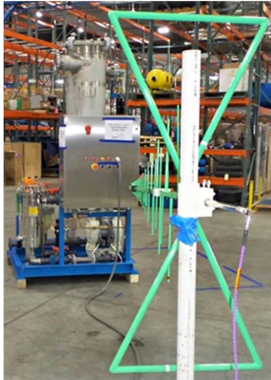
Figure 6: EMC compatibility testing of radiated emissions of a Rogers Engineered Vacuum System.
