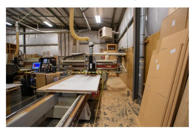
A critical component in their cabinet manufacturing process is a vacuum pump. The pump supplies vacuum to multiple hold-down tables. The vacuum suctions sheets of wood to a table while it is precisely cut into cabinet panels.
