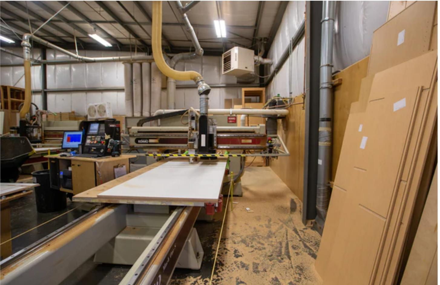
A critical component in their cabinet manufacturing process is a vacuum pump. The pump supplies vacuum to multiple hold-down tables. The vacuum suctions sheets of wood to a table while it is precisely cut into cabinet panels.
