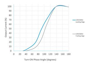
Note: Operating the driver below the minimum Turn-On Phase Angle can result in driver output turning off or unstable performance.
