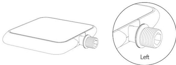
The left pedal is further identifiable by a groove / letter on the pedal collar.
