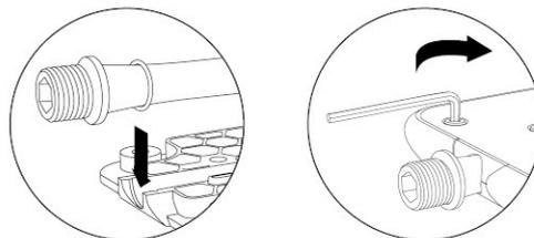
Fitting O-ring into designated grooves and tightening half-shells.
