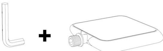
An 8 mm Allen key is needed to mount the pedals on the crank arms.
