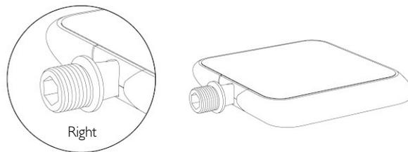
Attention! The right pedal has a right hand thread and the left pedal has a left hand thread at the pedal shaft for mounting on the crank arm.
