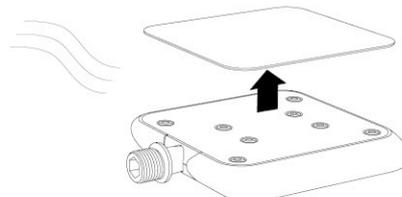
Apply heat with a hair dryer in order to remove Griptape.
