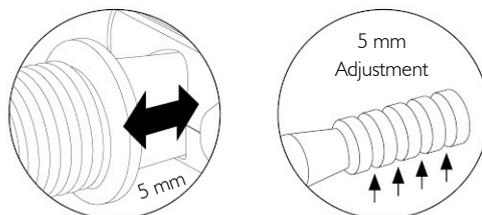
Distance between platform and crank arm can be extended or reduced by 5 mm. To adjust pedal width, unscrew half-shells and change position of the pedal shaft; see also maintenance. This provides additional space for large shoes.
