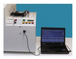
Laptop to the degausser and open the logging program. Click on the "Find Machine" button and all the unit details are automatically entered into the log including model, serial number and firmware version. Further data regarding operator, customer and media is then entered via keyboard (or optional barcode scanner).
