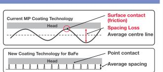
Smaller undulation with small and uniform protrusions reduces output fluctuation, resulting in less noise.
