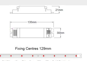
The ADM/1/LEDS16 is supplied as a complete non-maintained DALI self-test emergency driver/LED strip for integral mounting within a luminaire.
