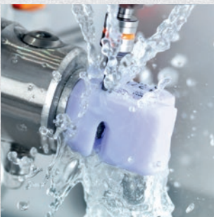
"Carving Mode" - excess material is being cut off as a whole
