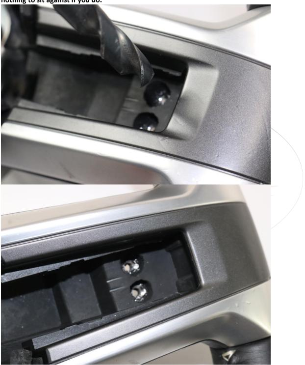
Step 6: Mount the screws and bracket from the back side, hand tighten the 6-32 nuts from the inside of the steering wheel. Tighten nuts and bolts.
