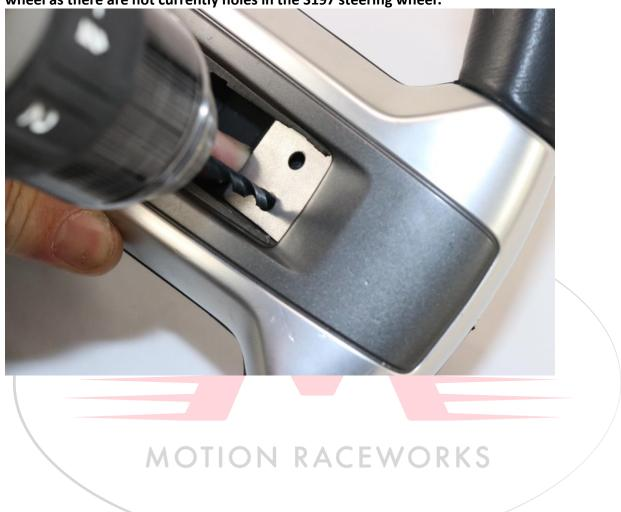
Step 5: Remove drill guide. Come back and use a ½" drill bit to open the rubber portion on the inside large enough to accept the nyloc nuts so that they recess down into the rubber. DO NOT DRILL ALL THE WAY THROUGH THE ALUMINUM during this step as the nut will have nothing to sit against if you do.
