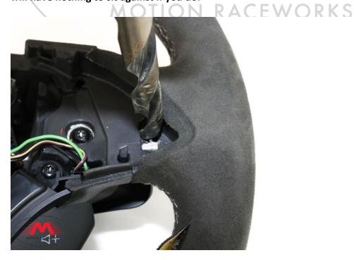
Step 6: Mount the bracket by running the stainless button head bolt from the inside of the wheel and threading into the bracket on the back side.
