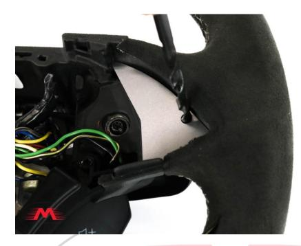
Step 5: Remove drill guide. Come back and use a ½" drill bit to open the rubber portion on the inside large enough to accept the button head screws so that they recess down into the rubber. DO NOT DRILL ALL THE WAY THROUGH THE ALUMINUM during this step as the bolt will have nothing to sit against if you do.
