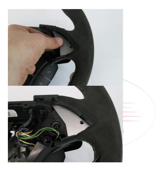
Step 4: Use 7/32 Drill to drill from the inside of the steering wheel outward (drilling perpendicular to the drill guide), this will give proper orientation and lineup of screws for the button bracket to sit correctly on the steering wheel as there are not currently holes in the 16-18 steering wheel.
