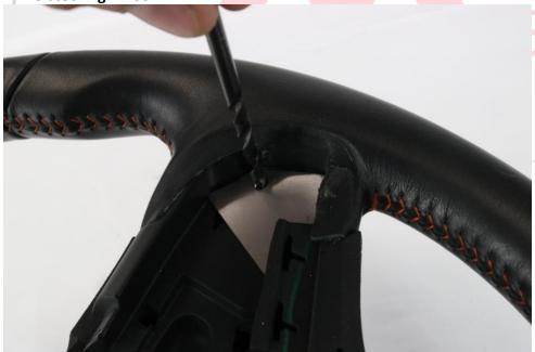
Step 5: Remove drill guide. Come back and use a ½" drill bit to open the rubber portion on the inside large enough to accept the button head screws so that they recess down into the rubber. DO NOT DRILL ALL THE WAY THROUGH THE ALUMINUM during this step as the bolt will have nothing to sit against if you do.
