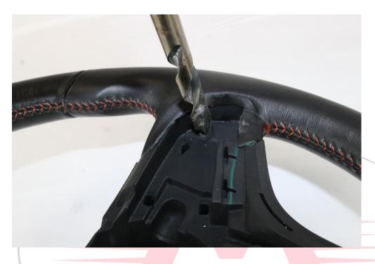
Step 6: Mount the bracket by running the stainless button head bolt from the inside of the wheel and threading into the bracket on the back side.
