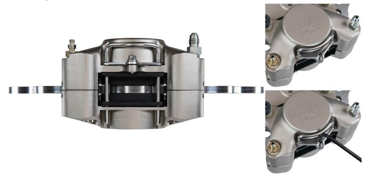
**Step 7:** If there is pad to rotor contact, determine which side is causing the interference. Shim the caliper or the bracket as needed using the supplied shim kit to center the caliper and ensure the caliper is parallel to the rotor. \*\*What is required for one side of the car may not be the same as the other side. Check each side individually\*\*
