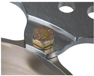
**Step 3**: Place the caliper bracket on the face of the knuckle as shown below. Apply red Loctite to the M12 X 1.75 X 40MM hex bolts and tighten to 60ft/lbs.
