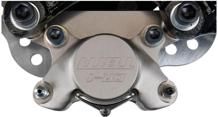
**Step 6:** Remove the pad retainer bolt (if already inserted). Insert the brake pads from the top of the caliper and reinsert the pad retainer bolt. Hold the pads against the caliper housing. Spin the rotor assembly to check for contact between the rotor and brake pads. There should be no contact between the rotor and pads. Be sure to tighten the pad retainer bolt once pads are installed.
