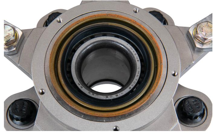
**Step 6**: Mount the caliper bracket using the 3/8-24 x 1 3/4" FHCS and then torque to 37ft/lbs.
