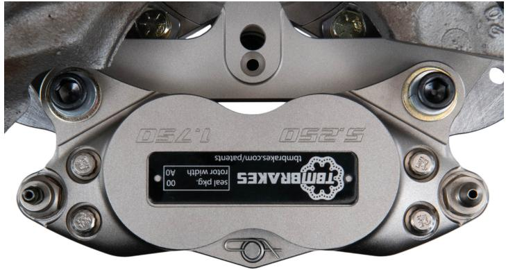
**Step 9:** Remove the pad retainer bolt (if already inserted). Insert the brake pads from the top of the caliper and reinsert the pad retainer bolt. Hold the pads against the caliper housing. Spin the rotor assembly to check for contact between the rotor and brake pads. There should be no contact between the rotor and pads. Be sure to tighten the pad retainer bolt once pads are installed.
