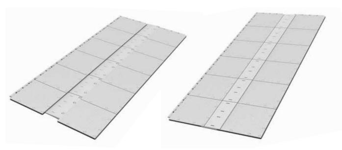
**Step 3:** Lay a fresh row of panels along the edge of the ramps. The male edge of the panels will face the ramps with the female or leading edge facing the direction of the build.
