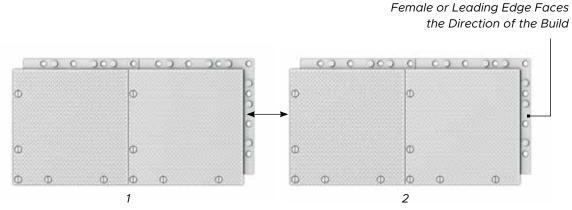
Note: Panels are properly aligned when the surface of the second mat is flush with first panel.
