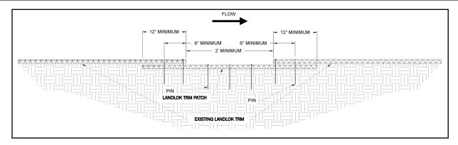
Figure 22: LANDLOK Patch Cross Section
