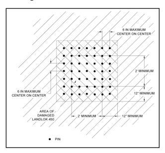
Figure 23: LANDLOK Patch Plan View
