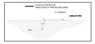
Figure 5: Initial Channel (IC) Trench Placement
