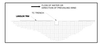
Figure 18: Terminal Channel (TC) Trench Alignment
