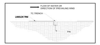
Figure 19: Terminal Channel (TC) Trench Placement
