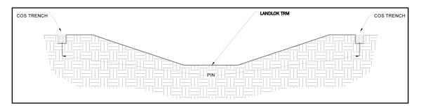
Figure 17: Crest of Slope (COS) Trenches Complete
