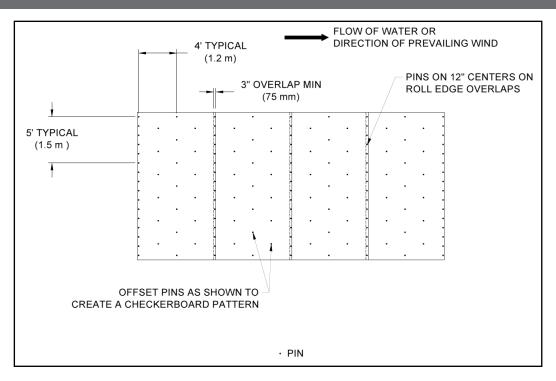
Figure 13: Example Edge Overlap Pattern
