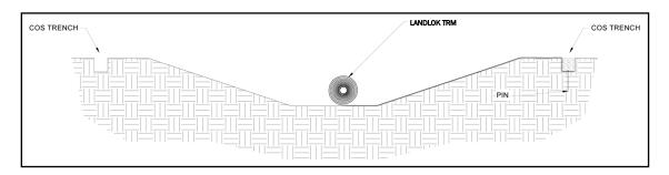
Figure 11: Perpendicular Placement of LANDLOK across Channel
