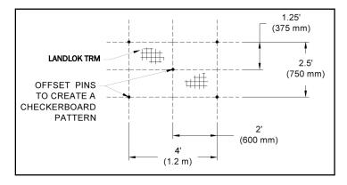
Figure 12: Example Pin Pattern
