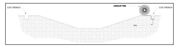
Figure 10: Crest of Slope (COS) Trench Placement
