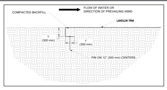
Figure 3: Terminal Channel (TC) Trench
