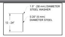
Figure 6: Securing Pin
