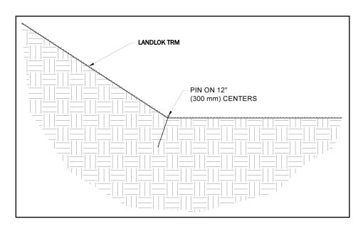
Figure 16: Break in Slope Interface
