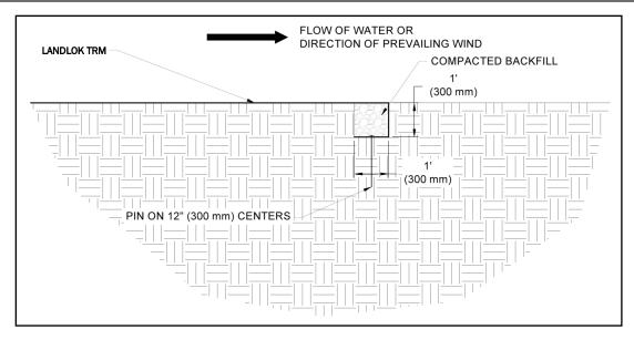
Figure 1: Initial Channel (IC) Trench
