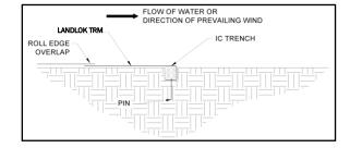
Figure 7: Initial Channel (IC) Trench Complete
