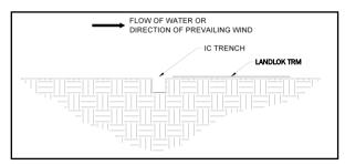
Figure 4: Initial Channel (IC) Trench Alignment
