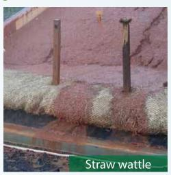
Staking, weight, and level surface are primary drivers in sediment removal performance. More staking on straw wattles creates more low points, which are more likely to overtop.
