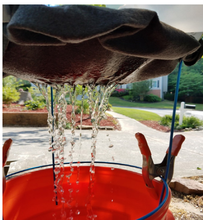
Figure 6 - class 1 nonwoven Figure 7 - class 1 woven
