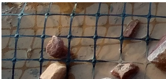
Figure 4 - Geogrid aperture size
