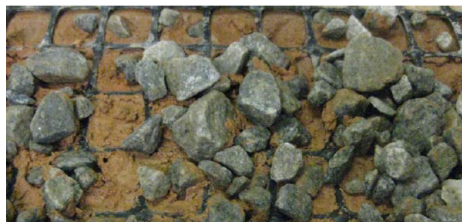
Figure 5 - Geogrid aperture size
