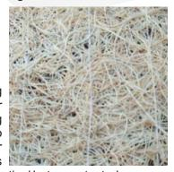
Curlex NetFree ECB is intended for use in low-flow channels. Large scale testing that followed procedures outlined in ASTM D-6460, "Standard Test Method for Determination of Erosion Control Blanket (ECB) Performance in Protecting Earthen Channels from Stormwater-Induced Erosion", showed the ability of Curlex NetFree to protect channels from stormwater-induced erosion. Curlex NetFree will withstand tractive forces  $\leq 1$  lb/ft².
