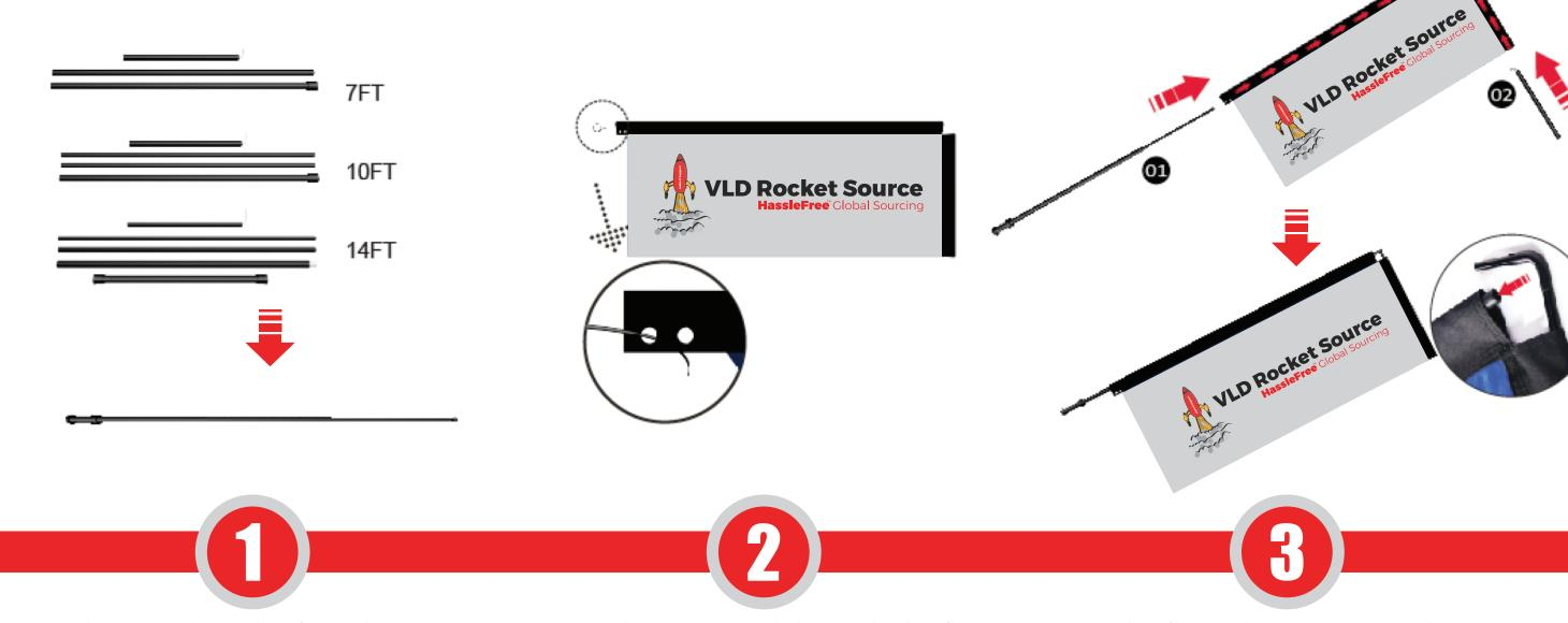
Join the upright poles from largest to smallest - simply insert one end of the poles into the other and push them together. String bungee cord through the flag grommet.
