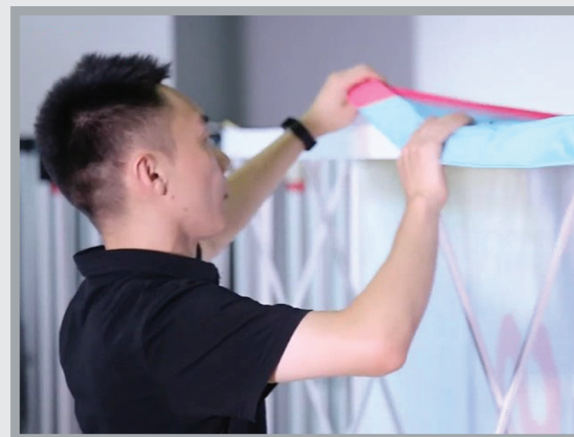
Each side is with Velcro. Start attaching the graphic to the frame with Velcro on one side and move forward to the next.
