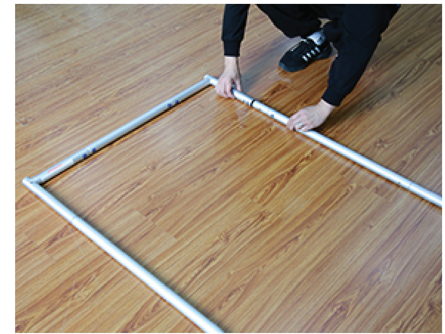
Press the push pin grip and lock the sections of the stand in place.
