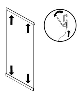
Insert both graphics edge into the snap-rails.
