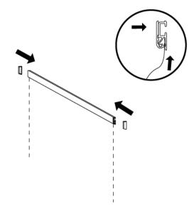
Slide the top of the graphic under the end-cap and close the end-cap to secure the graphic. Remove the plastic end caps from the upper beams.
