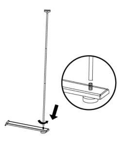
Insert both the 3-piece-poles into the hole of the base, then fix the other end of the base unit. Connect the two basic unit with a pole.
