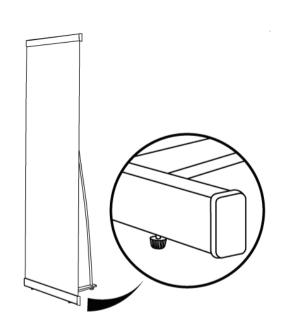
The unit can be levelled by adjusting the threaded feet at the bottom of the base unit.
