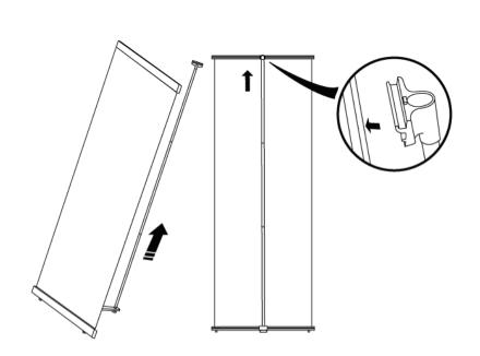
Adjust the graphic into the right position with a special unit. The hook at the top of the pole slips into the rear slot of the banner beam. A marker on the beam indicates the beam's center where the pole should be inserted.
