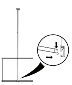
Take fix of the bottom pole with the special unit then spread the graphic to the top of the 3 piece pole.
