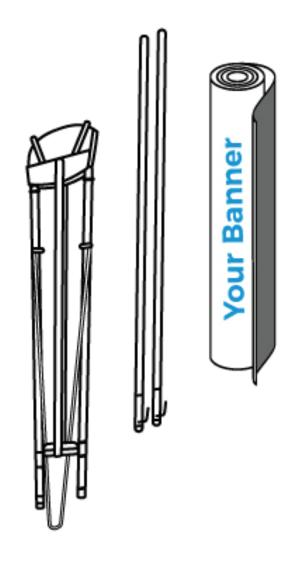
Material preparation. Secure the tripod base on level ground.
