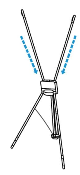
Insert the arms with the hooks into the tripod facing forward.
