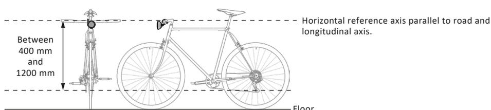
Horizontal reference axis parallel to road and longitudinal axis.
