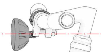
① Apply handlebar adapter to adjust diameter if needed. (35.4 mm to 31.8 mm).
