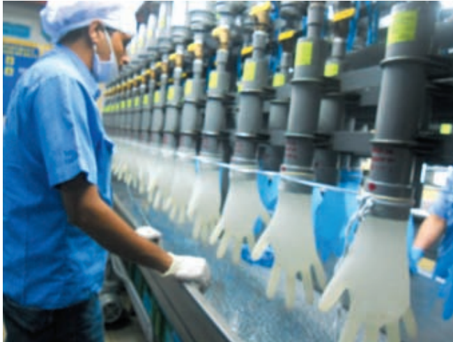
The gloves undergo 1000ml water-tight testing in strict compliance with ASTM D3578 (01) Standards.
