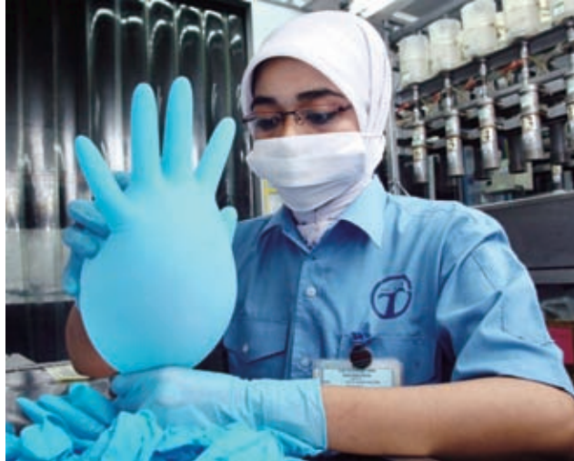
Visual inspection of the gloves is carried out to ensure high quality and reliability.
