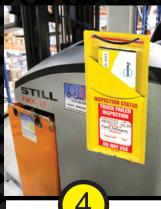
If equipment fails inspection its immediately tagged out of service with notes ready for maintenance
