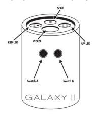
**Power On:** hold switch-A for 1 second. When the torch switches on, the power indicator light will come on.
