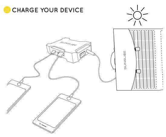
Once the junction box is powered, the red LED indicator should turn on. You can now connect your laptop, smartphone or any other device to the special junction box's USB-A or USB-C port.
