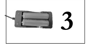
Charge the batteries until the charger indicator lights turn green. NOTE: On first-time charging this can take up to 6 hours or more
