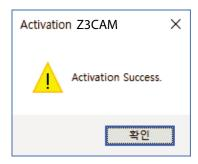
If nothing happens during the Z3Cam Sensor Activation, you can activate it another way. Go into your C:Drive > Open "Z3CamSensor" > Open "Z3CAM\_Activation." > Browse for the license file.
