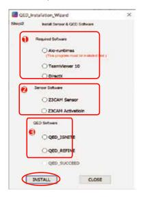
Please install each software one at a time ONLY. Click "Install" button for each install. "Aio-Runtimes" must be installed first. Go to next page for steps.
