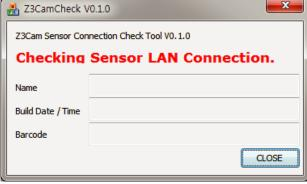
Make sure the Sensor LAN connection is good before the software installation process.
