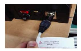
Take out all 3 components of the power source: power cable, power adapter, and power connector. Connect all 3 accordingly and connect the "Power Connector" end directly to the sensor as shown below. Turn on red switch.
