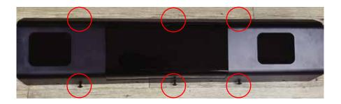
Slide the sensor bar with the 6 screws up and over through the bracket hinges. Make sure the screws are secured in the hook part of the hinges. If the screws do not go into the hinges, adjust by tightening the screws just a little.
