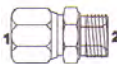
ADAPT FEMELLE JIC 37° TOURNANTE / MALE BSPP ADAPTER FEMALE JIC 37° SWIVEL / MALE BSPP
