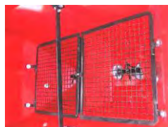
Strong net to filter possible fertilizer clots
