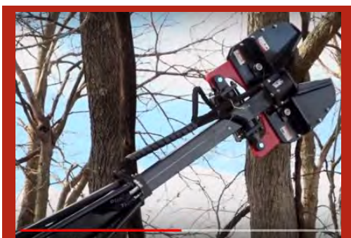
Model TC6451 Telescopic Clipper head with 36" telescope. Ideal for clean-up along ditches and waterways.
