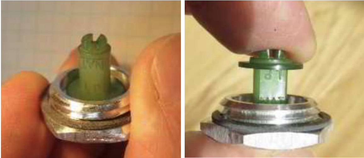
Natural gas (NAT) position
