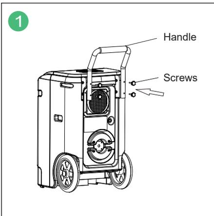
Put the handle into the groove at the back of the dehumidifier, making the 4 screws correspond to the screw hole.
