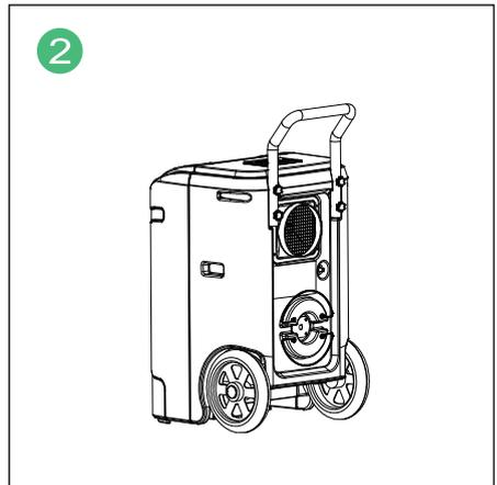
Tighten all the four hand screws, complete the installation.
