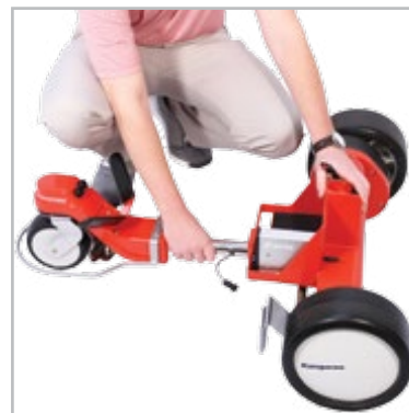
Steering Structure being inserted into chassis.
