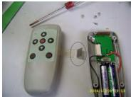
5. Question: The caddy does not respond well to the remote control handset? **Reply**: Please check the condition of the handset batteries. Make sure you don't exceed the range distance limit.
