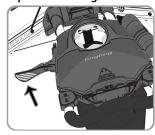
Pull upward to engage the parking brake and push down to release the parking brake.
