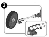
Install the rear wheels by pressing the "PRESS" button and inserting the axle of the wheel into the cart until the wheel clicks into place.
