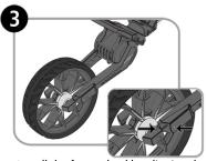
Install the front wheel by aligning the STAR on the wheel axle and the front fork of the cart and slide the front wheel into the fork blades until it clicks and locks into place.
