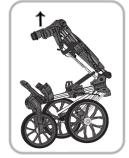
With the cart on the ground, pull sharply on the upper bag bracket and lift the Nitron until the cart fully opens.
