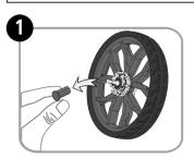
Remove the black plastic cap from the rear wheel axles.
