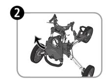
Flip the gray Handle Release Lever and adjust the handle to the desired height. Close the lever to lock the handle into position.
