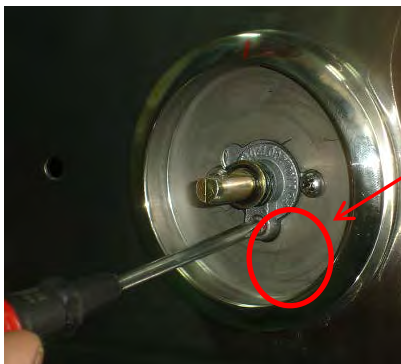
Low flame setting screw (where applicable)
