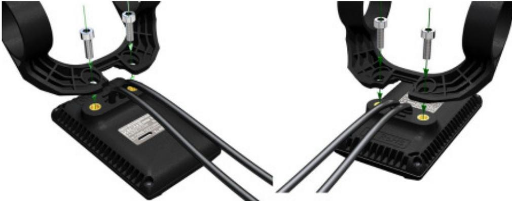
Clamps suit for 3 size of handlebar, 31.8mm, 25.4mm, 22.2mm, there are transfer rings for 25.4mm and 22.2mm, transfer ring must be assembled with the special directions, pay attention to the green arrow below.
