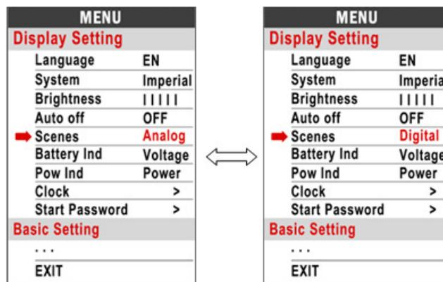
**8.6 Battery Ind** : Press UP/DOWN button to change the battery indicator, Voltage / Percentage / OFF.
