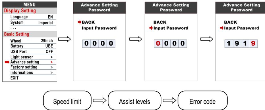
**8.15 Speed limit** : Press UP/DOWN will change speed limit, range 10km/h~45km/h. Default value is 25km/h.
