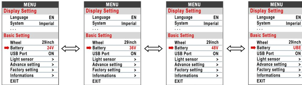
8.12 USB Port: press **UP/DOWN** level, select pres **OFF/ON**, Will be no Voltage/Current output after switching off.
