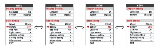
**8.12** USB Port: press UP/DOWN level, select presOFF/ON, Will be no Voltage/Current output after switching off.
