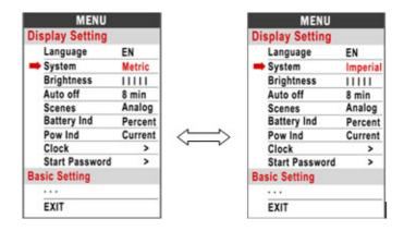
**8.3 Brightness**: Press Up / Down button to change the brightness of the backlight, I is darkness, IIII is brightness, default value is I.
