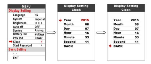
Note: There is an battery inside to sustain clock working when display is powered off, the battery can be charged when display is power on (riding). Battery often be exhausted after long time unused (after winter or transportation), you need to recharge the battery as below.
