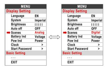
**8.6 Battery Ind**: Press UP/DOWN button to change the battery indicator, Voltage / Percentage / OFF.
