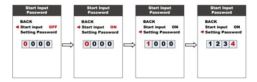
You need to input the right password before start with 30 seconds, display will power off automatically if the password was wrong.
