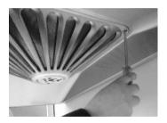
Align the Phillips screwdriver wit the screw hole and raise it upward forcibly meanwhile rotating it counter–clockwise about  $120^\circ$ , so as to remove the screw out of the cross slot of the exhaust fume collecting hood.
