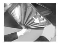
Hold the two screws on the filter mesh and pull it down to detach the two prongs inside from the exhaust fume collecting hood. Then pull the filter out in the arrow direction to remove it.
