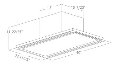
FALSE CEILING CUT: 21 13/20 " x 38 1/2" \*Can be installed up to 10 feet.
