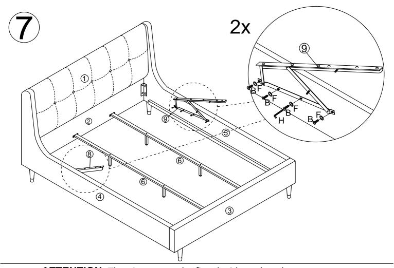
ATTENTION: The piston must be fitted wide end to the top as shown in the Assembly Instruction. Do not overtighten the nuts.
