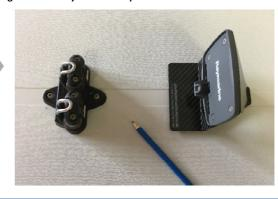
Step 4 - Remove the backing from the mounting pads.
