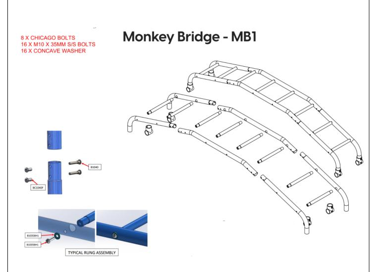
STEP 1: Assemble the left and right sides as shown with washers and bolts. DO NOT TIGHTEN
