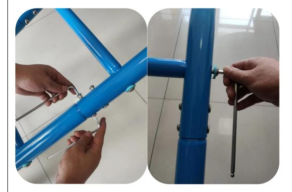
STEP 6: Evenly tighten all bolts. The frame may twist slightly which is normal, it will straighten during installation.
