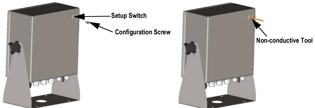
Figure 3-1. Setup Switch Location (Universal Enclosure)
