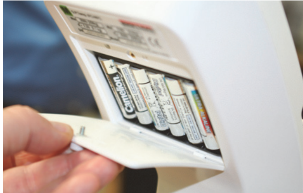
Figure 3-7. Batteries in Battery Chamber
